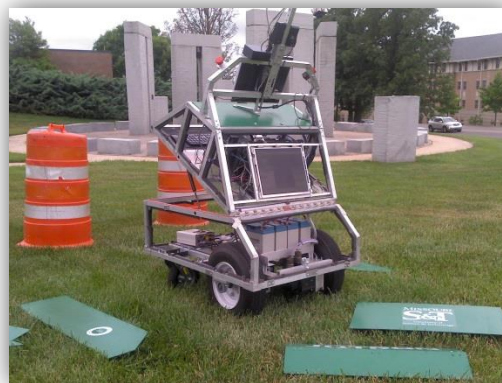
Figure 4.1.2: The Lexan panels of the shell removed from the robot
